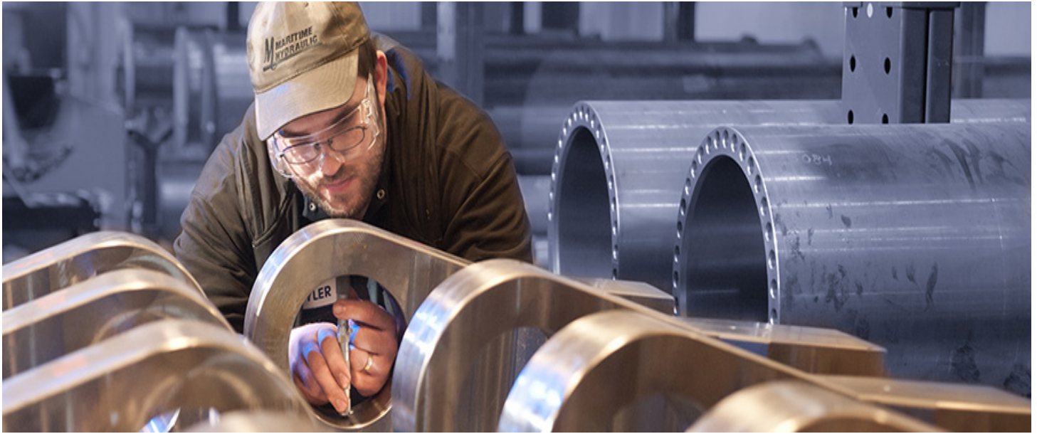
Final dimensional inspection of hydraulic cylinder components prior to assembly.
